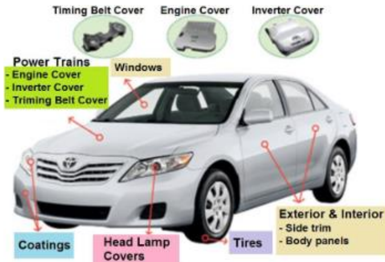
Fig 1-6: Components a vehicle from fiber composite material
