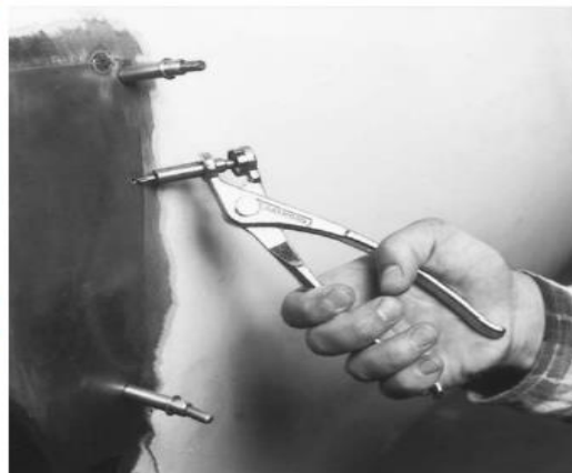
B These spring-loaded rivets can be installed and removed easily. They are ideal for holding panels together while welding.
