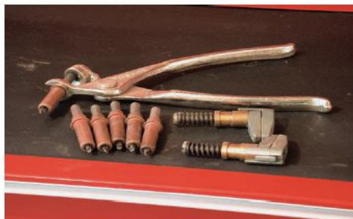
A These spring-loaded rivets and clamps can be installed and removed easily using special pliers. (Courtesy of Eastwood Company, www.eastwood.com)
