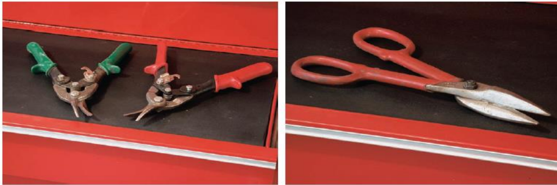
A Sheet metal cutting pliers come in right- and left-hand configurations for cutting in different directions.
