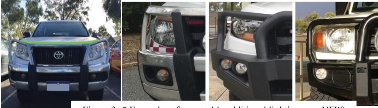
Figure 2- 5 Examples of acceptable additional lighting on a VFPS
