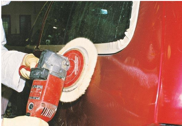
Figure 1-0-1 Polish the paint surface
