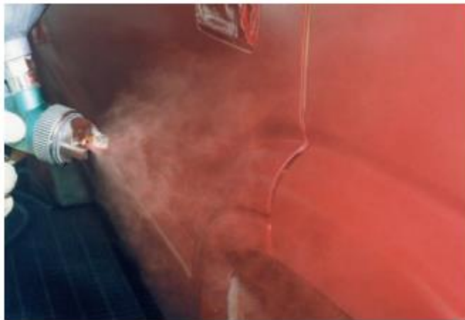
FIGURE 2.1. A spray gun is designed to atomize liquid material into a fine mist
