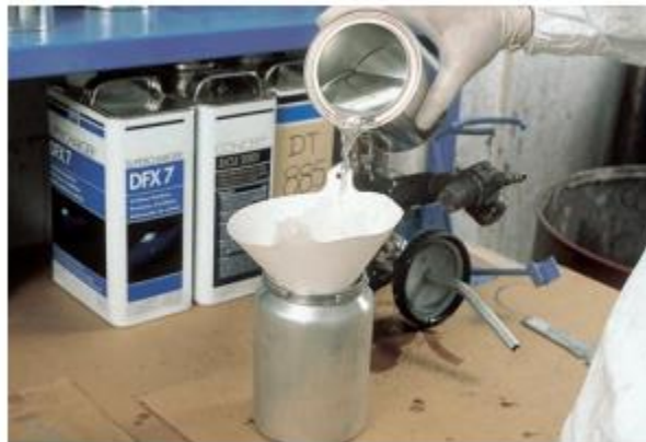
FIGURE 2.4. Always filter or strain anything you pour into your spray gun cup
